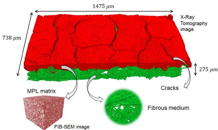
Figure 6. 3D digital image of GDL combining X-ray Tomography (fibrous medium, cracks) and FIB-SEM (MPL matrix)
