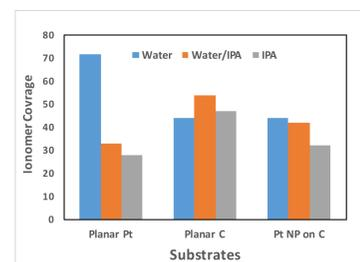
Figure 2. Effect of dispersion media on ionomer coverage on different substrates.
