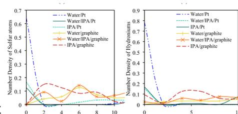
Figure 3. Abundance of sulfonic acid groups (a) and hydronium ion (b) at the substrate ionomer interface [1]
