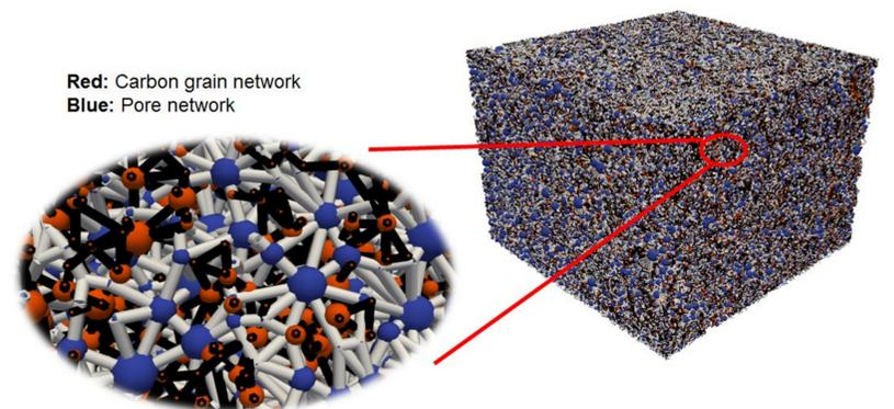
Figure 7. Pore and Carbon grain network extracted from a MPL matrix 3D FIB-SEM image using Porespy / OpenPNM
