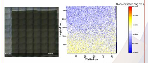
XRF of high-low graded ionomer content MEA
